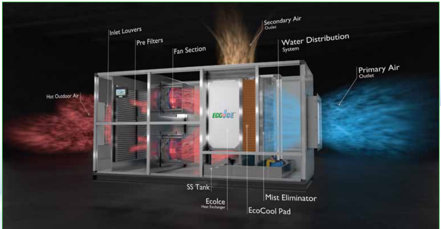
Fig. 7: Indirect-Direct Evaporative Cooling (IDEC) System Internal View
